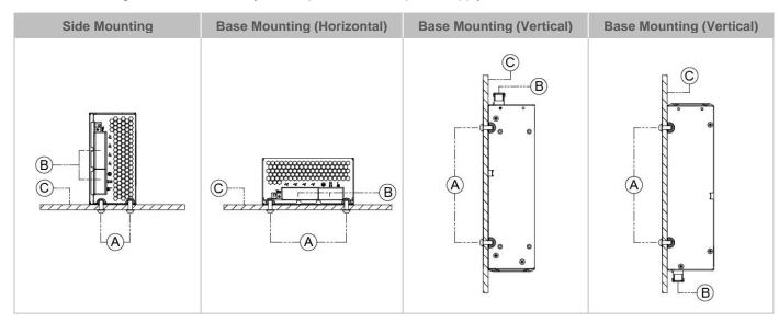
Fig. 2 Mounting Orientation
