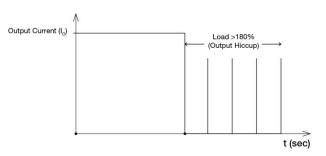
It is not recommended to prolong the duration of Io when it is <180% but >100%, since it may cause damage to the PSU.
