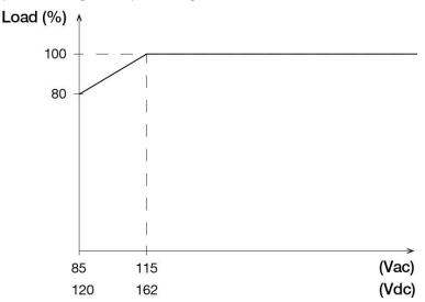
Output de-rating is required at 85Vac to 115Vac or 120Vdc to 162Vdc.
